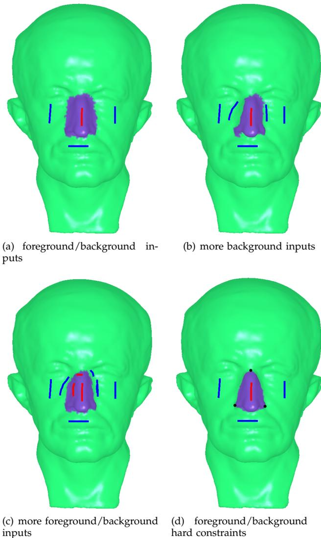
Fig. 9. While gradually inputting more foreground and background strokes does not guarantee a nice cutting (a-c), specifying three hard constraints at the weak boundary can help to quickly find a satisfactory cutting (d).
