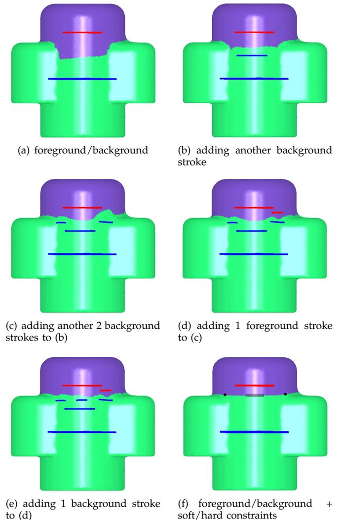
Fig. 10. (a)-(e) show the cutting results by gradually adding foreground/background strokes. (f) shows the result by inputting some soft/hard constraints in addition to the initial foreground/background, which is a satisfactory result reflecting user intention and human shape perception.
