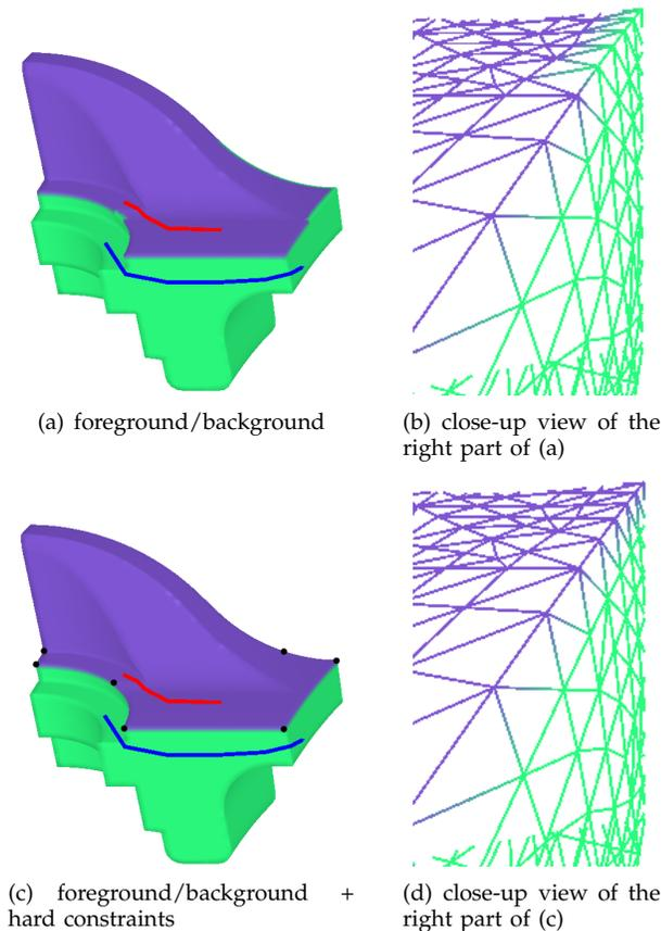
Fig. 2. Specifying a few points (hard constraints) on the desired cutting contour helps the random walks find more accurate results.
