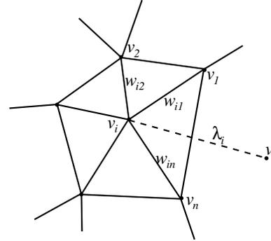
Fig. 3. A vertex  $v_i$  with the soft constraint can be considered to have a virtual neighboring vertex  $v$  with the probability of  $1/2$  connected by a virtual edge of weight  $\lambda_i$ .
